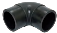
90° ELBOW PE100 SDR 11 - Water PN16 / Gas 10 Bar SDR17 - Water PN10 / Gas 6 Bar SDR 7.4 - Water PN25 SDR 9 - Water PN20 d20-500
