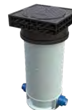
SERIES 80/32-200 Fixed height surface box for service connection valves Square top Cast iron lid PA+ body
