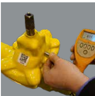
MINIMUM COATING THICKNESS
